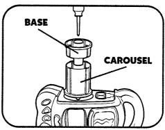
2. Remove photo carousel from compartment. (Note: Batteries may also slide out of their compartment.) Use a Phillips screwdriver to loosen screw attaching base to carousel (screw will remain attached to base).
